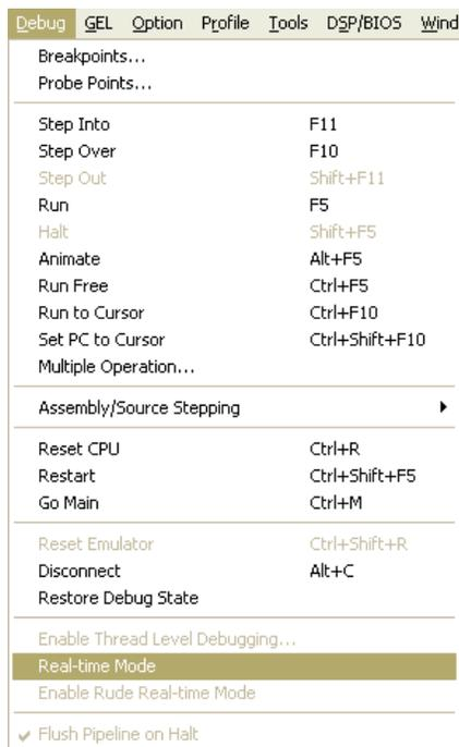
**Figure 6. Real-time Mode Option in the Debug Menu**
